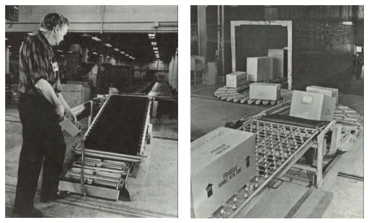
Installed as a fixed conveyor extension unit, one man can effortlessly "walk" the unit into a van stationed at any of three loading docks. There is no time lost when a truck has been emptied and another has not yet come into that dock. The operator simply leads the UPC into the truck in an adjacent dock and unloading begins again in seconds. When not in use, the entire UPC stores under the fixed conveyor system.
