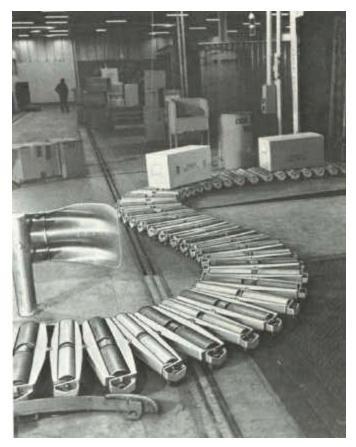
The UPC's versatile "snaking" capability enables effortless handling of luggage, packages, etc. through cramped transport routes, thus reducing loading/unloading time and employee fatigue.
