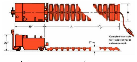
A Lengths are available up to 175 FeetB Model UPC26-26", Model UPC49-49"
