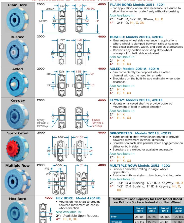
NOTE: HI: High-Impact Plastic, X: Synthetic Rubber Coated Polypropylene Rollers,
