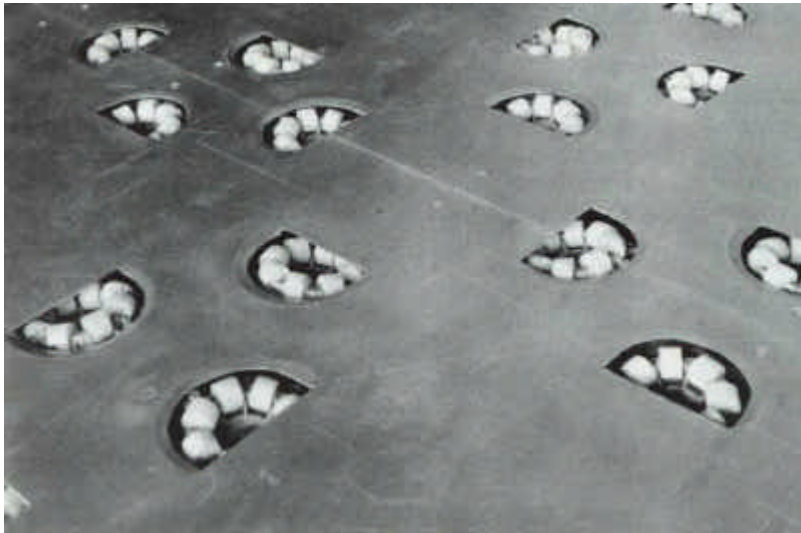
Remote Controlled x, y and Rotary Movement of heavy loads in a powered Transdisc® system with a cover plate.
