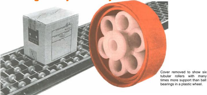
Superwheel can be interchanged with standard skatewheels. It weighs only .057 lbs per wheel and can reduce the weight of a typical gravity conveyor section by 40% or more.
