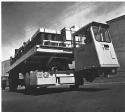
*Karry-All accepts, transports and discharges crated or skidded loads up to 7 1/2 tons in seconds; all functions are driver controlled. The cab swings to side permitting head-in approach to loading dock. Truck deck elevates to match conveyor on the dock. Conveyorized truck deck discharges half of full load. Deck also tilts for gravity discharge. Travel is at highway speeds.*
