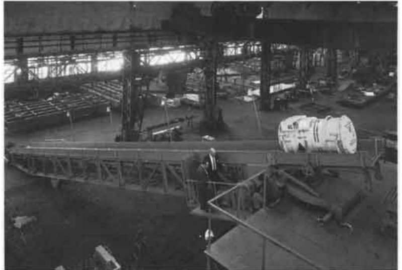
Missile Guidance Capsule fastens to metal belt for secure travel. Head section pivots downward for transfer to bed of special shipboard transporter. Pivoted, rotating and traveling head and tail mounts compensate for drift, roll, pitch and buoyancy of the ship.
