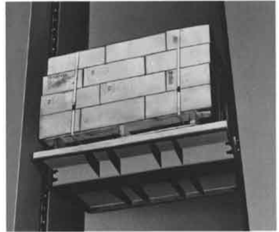
Vertiflo can deliver 4000 lb pallet loads at a 4 per minute rate.
