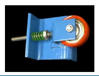
The Rollerslo® RXC141 is designed as a heavy-duty version with a more accurate adjustment and higher spring tension. The higher spring tension gives the RXC141 the ability to act as a brake as well as a flow controller. Several RXC141's would be used along the length of the roller conveyor to control the speed of the object.
