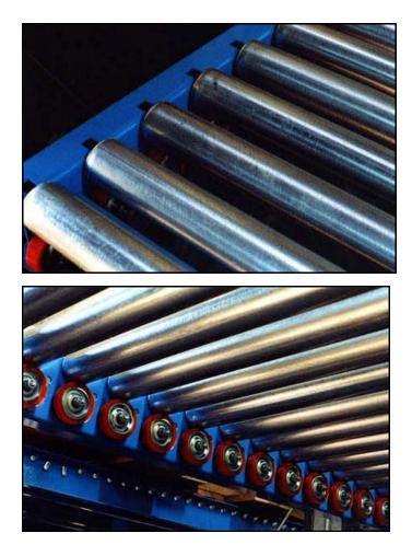
Rollerflo® can handle plastic pallets, wood pallets with very few and or extremely narrow runners as well as a wide variety of sizes and shapes of loads. Rollerflo® conveyors are roller conveyors with a difference! They utilize the hysteresis control principle of Kornylak's patented Palletflo® urethane coated skate wheels.
