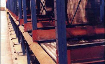
High hysteresis Palletflo® wheels are used for the necessary speed-retarding action. These urethane coated heavy duty skate wheels are resilient enough to allow the rollers to handle some degree of irregularity in the bottom of the pallet, or can.
