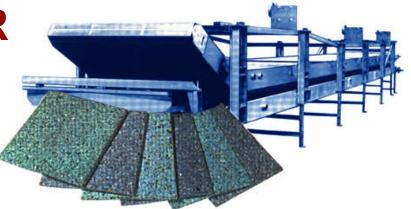
flexible polyurethane salvage into a high value carpet underlayment for which there is a steadily growing market that is as large as the carpet industry itself. This continuous process eliminates as much as 50% of the labor in older methods and reduces waste and regrind by as much as 95%. Film or backing is applied "on the run," and the finished product is automatically compressed, as it is rolled up, wrapped and sealed in standard lengths at the end of the line.
