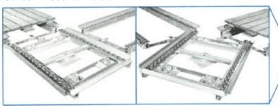
The Turntable is a simple device that makes it easy to change directions of the flow lines or divert the pallet to one of several intersecting lines. It rotates on lubricated roller bearings to minimize turn effort. A quick-acting Stop aligns the turntable with either line and locks it during transfer. The Stop is foot-operated for convenient release.
