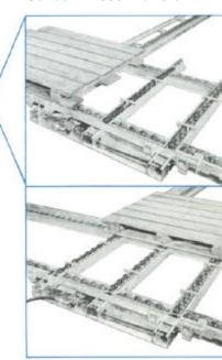
The Transfer is utilized where you want movement at right angles to the mainline but without pallet rotation. A footcontrolled valve raises the Transfer rails, and an easy push discharges the pallet to the branch line, which is 3/4" higher than the main line.
