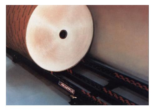
A special application of Palletflo for flowing paper rolls is being test and video recorded for a customer.
