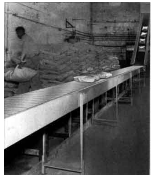
Positive belt tracking and smooth surface of Armorbelt permits easy side loading and unloading of heavy bags.
