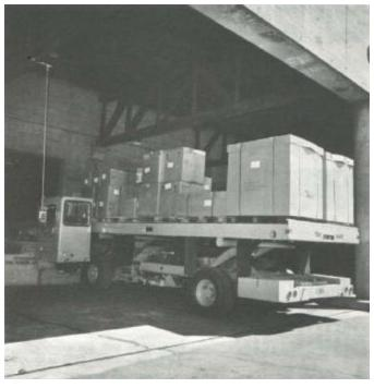
AUTOMATIC UNLOADING in seconds: Karry-All driver starts dock-side conveyor, using controls outside cab widow. Powered rollers on Karry-All cargo deck swiftly transfer load. All operations are controlled from the cab.
