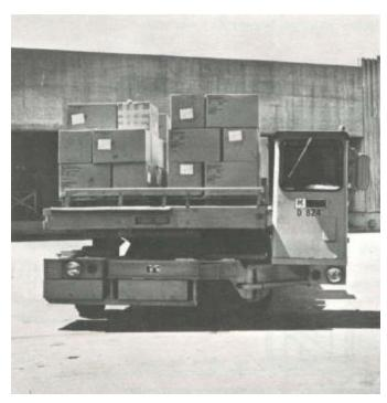
APPROACHING DOCK, driver operates controls to swing his cab aside and to elevate Karry-All cargo deck for perfect line-up with obckside conveyor. He will then lower the cargo restraining bar, clearing the way for unloading.
