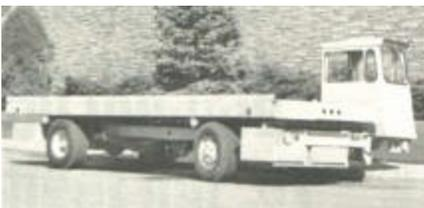
The vehicle is capable of speeds of 50 mph and can be driven with the swing-away cab in front, at the side, or any position between, road conditions permitting.
