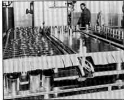
Smooth in-line accumulation gives canned shortening a 12 minute unagitated hardening period.
