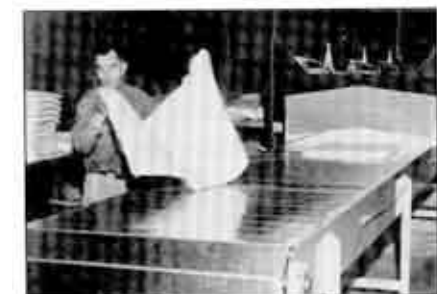
Reflective heat resistant Armorbelt on this automotive topper line is easy to clean of spilled latex cement.
