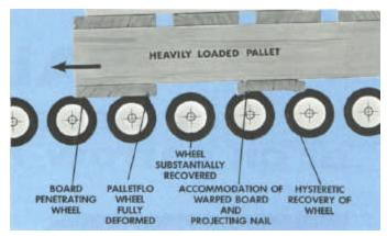
Palletflo wheels deform to accommodate any standard pallet. Hysteresis in each controls pallet speed.
