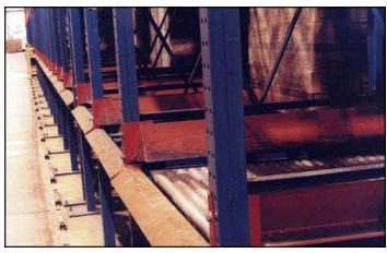
Rollerflo® can handle plastic pallets, wood pallets with very few and or extremely narrow runners as well as a wide variety of sizes and shapes of loads. Rollerflo® conveyors are roller conveyors with a difference! They utilize the hysteresis control principle of Kornylak's patented Palletflo® urethane coated skate wheels.
