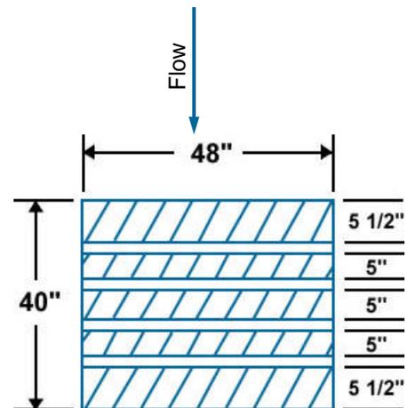
Example of how diagram at left should be marked up to show bottom boards.
