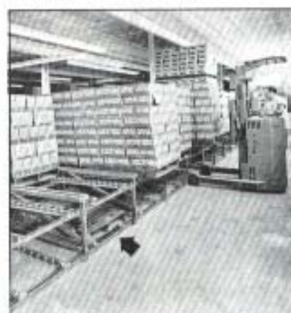
When an empty pallet returns to the rear of a Palletflo order picking rack, it is easily removed by the same truck which replenishes the rack. This entirely eliminates manual handling of heavy pallets in the Palletflo system.
