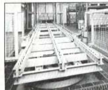
Turntable and Palletflo gravity conveyor serve an elevator in France.
