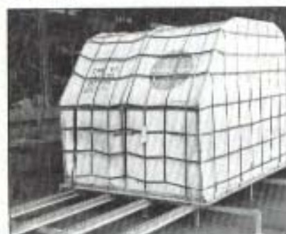
14,000 lb air cargo load rolls at controlled speed on Palletflo line. Aluminum pallet is gently supported on elastomeric Palletflo wheels with no indentation or scratching.
