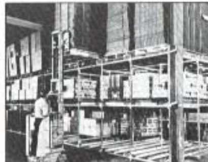
Last in - first out feature on top shelf allows access to shipping supplies from rear of a Palletflo order picking rack.
