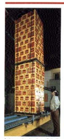
Assistance in planning a Palletflo installation at a European brewery resulted from this successful test using a 17 ft, high x 6400 lb. stack of bottle beer. The new installation permitted one tier operation and large unit load handling.
