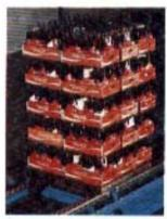
Cases of soft drink tested on Palletflo to confirm that the loosely stacked loads would roll smoothly at a controlled speed.
