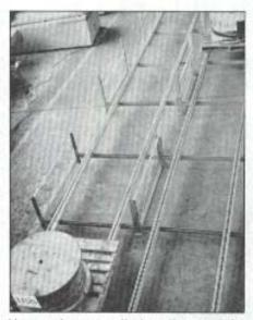
Hysteresis controlled pallet on right travels at steady 11 ft./min. Uncontrolled load on left reaches speed of 240 ft/min.
