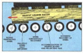
The tread of Palletflo wheels is resilient allowing the irregularity to ride through the wheel instead of having to climb over it. The result is a lower running slope and greater regularity in speed.
