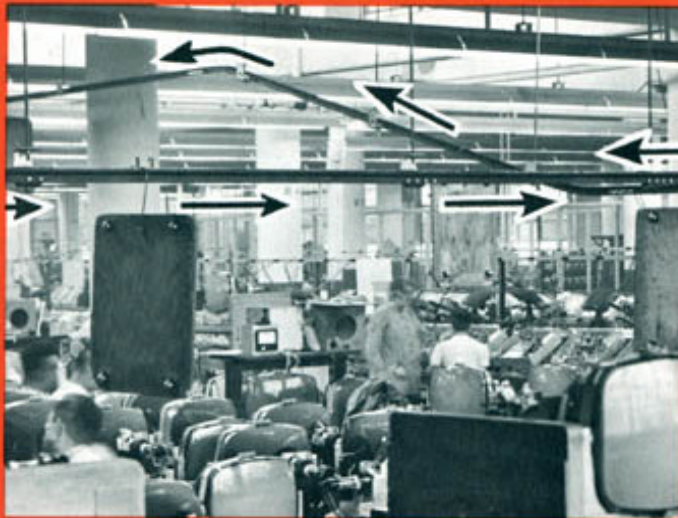
One-way Monoflo Conveyor returns "dollies," used for TV chassis assembly, to start off assembly line.
