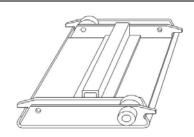
Two rollers mounted diagonally on each slat for stability and high load capacity. Long wheel brackets stiffen the slat.
